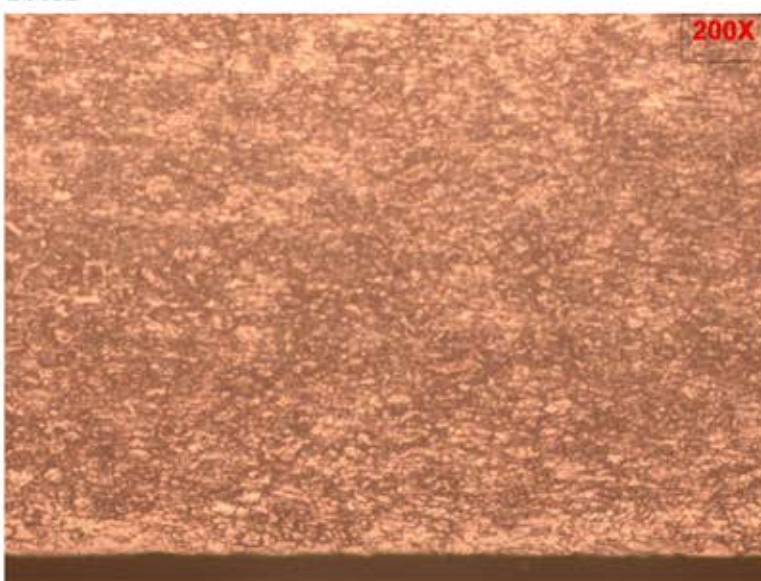
CROSS SECTION COPPER LAYER AS ETCHED 200X
